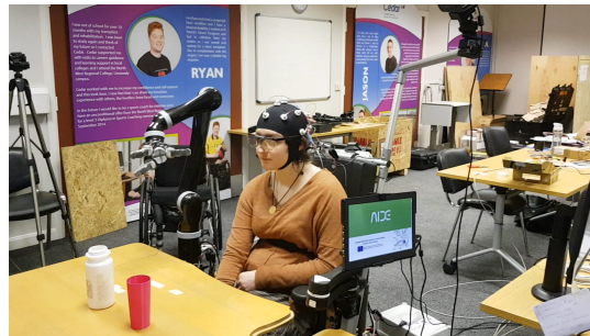
Final prototype tested on a patient affected by SLA
